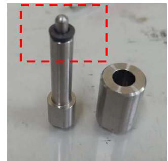
6. Be aware of the direction when installing sealing ring
