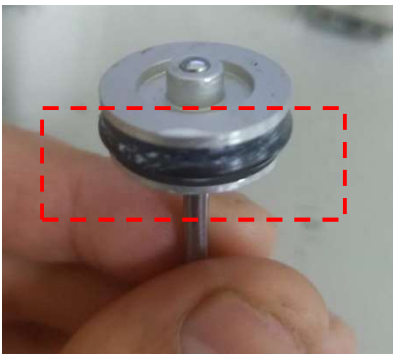
7. Wipe the firing pin with high speed maintenance oil
