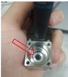
4. Clean the inside with alcohol and dust-free wiper
